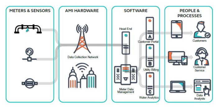
"Advanced metering infrastructure (AMI) is an integrated system of smart meters, communications networks, and data management systems that remote collection of meter data for billing and maintenance purposes allowing for immediate profitability and reliability."
