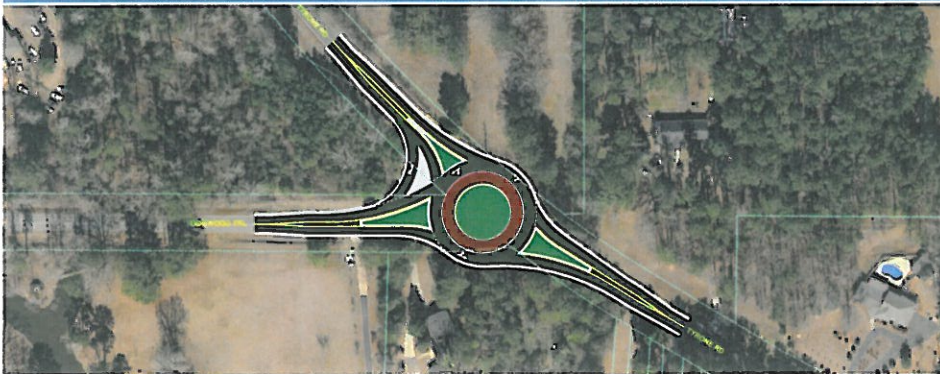
Graphic 4.11 - Concept: Intersection Improvement at Dogwood Trail - Roundabout
